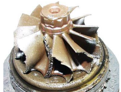
Foreign object damage due to hitting by larger metal fragments
