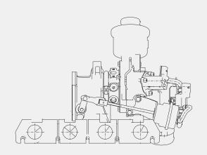
The 1.8 TFSI also uses a compact integrated turbocharger module. Since the manifold and turbine housing are combined to form a single component made of a highly heat-resistance material, this system not only saves space, it also offers thermodynamic advantages.
