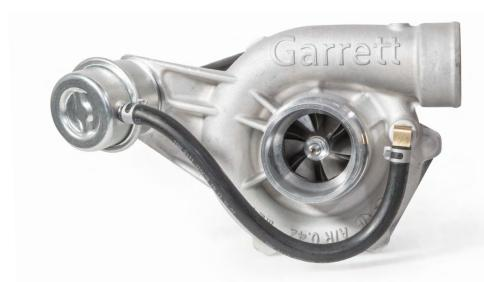
Garrett | Classic Turbo incorporates modern engineering with direct-fit installation for the iconic Lancia Delta HF Integrale 8V, 16V | Lancia Dedra | Alfa 155 2.0 Q4 | Fiat Coupe 16V. The modern journal bearing rotating group utilizes a 360-degree thrust bearing for improved reliability. Garrett integrated the actuator bracket into the compressor housing to strengthen the turbocharger. This turbocharger includes a gasket kit for a direct-fit installation.
